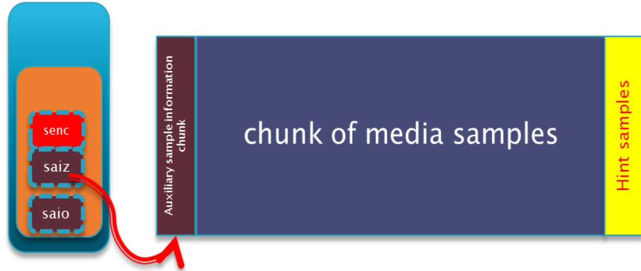
Figure 5.1 Encrypted Track structure - Storage of CENC related information.
